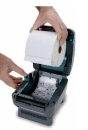
Make sure that the core is resting on the hangers and that the roll turns freely. The roll must not sit in the bottom of the media compartment.
